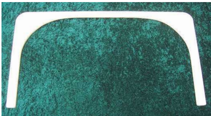
▲ Pic.9 The top rail made from 19mm ply
